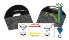
Mesoporous silica thin films are combined with redox-responsive ferrocene-containing polymers. The influence of chemical oxidation on the ionic accessibility shows a redox-controlled membrane gating as function of polymer location and pH value. This is a first step towards a redox-controlled ionic transport through nanopores, and thus towards fast, reversible, and external control of charge-selective membrane gating.
