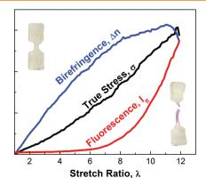
Simultaneous measurements of mechanical properties, birefringence and fluorescence images characterize the relationship between stress, polymer chain alignment, and activation of a force-sensitive chemical species centrally bonded into a polymer backbone.
