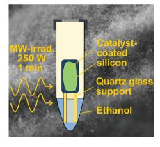
A fast microwave-assisted synthesis for the fabrication of square centimeter large free-standing carbon nanofibrous (CNF) films is reported. The obtained CNF coatings are about  $10~\mu m$  thin and exhibit a good stability and partial self-delamination from the substrate, which enables their detachment from the substrate without the need for further treatment. Morphologic investigations by scanning electron microscopy and a growth model are presented.
